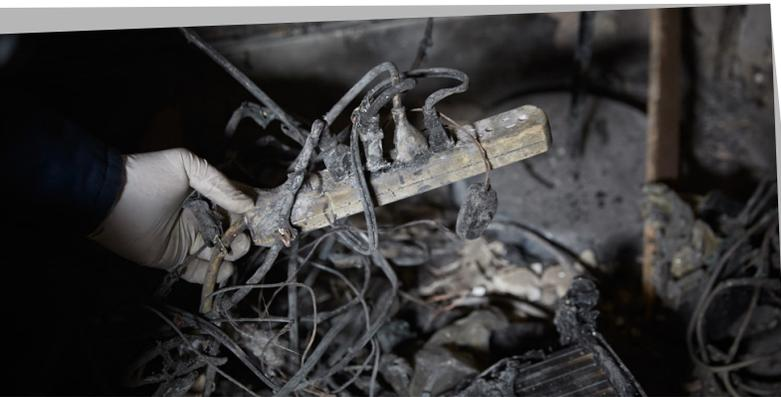
**Keep power bars and cords away from moist or wet environments.** Salt-water aquarium electrical should be installed by a professional to provide protection from moisture and contaminants. Normal power bars and extension cords will not do. Also keep weather-proofing covers closed on outdoor outlets.
