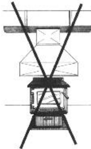
*CAUTION Never attempt to use a wood stove as a central furnace by putting a hood over it and connecting a furnace duct to the hood. This practice not only violates the building codes, it also disrupts the air-moving system and can cause the stove to spill smoke into the room. The biggest danger is the possible reversal of chimney flow that can quickly fill the house with carbon monoxide which can be hazardous.*
