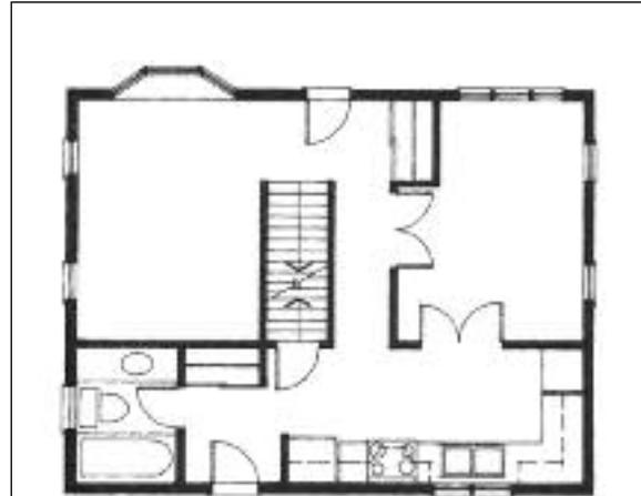
*A house like this, with spaces divided by walls, can be difficult to heat with a single space heater. A central heating furnace might be a better choice.*
