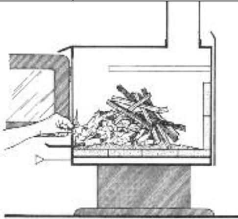
*This is the traditional way to start a wood fire. Use plenty of crumpled newspaper and dry, finely-split kindling. Set the air control fully open. Light the newspaper near where the combustion air enters the firebox. When a kindling fire is built properly, you should expect instant ignition and no smouldering.*
