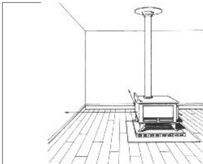
*The clearance for an uncertified radiant stove is 1200 mm (48 in.) and for a stove with a sheet metal jacket or casing the clearance is 900 mm (36 in.). The clearances are large because they apply to all shapes, sizes and designs of stoves that have not been tested to determine the actual clearances.*
