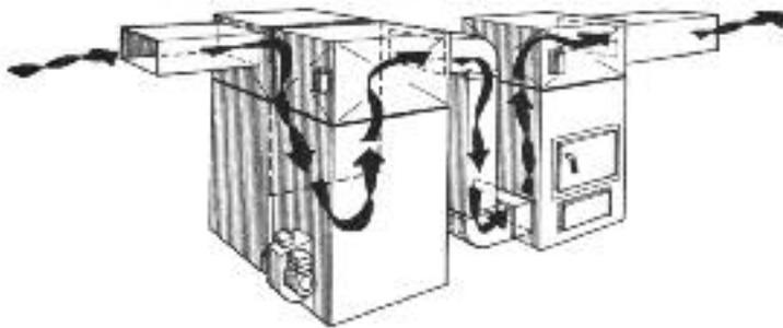
*The add-on is placed beside the existing furnace and special ducts are installed to connect the two units. Note that the air passes through the original furnace, then through the add-on and into the ducts for distribution to the house.*
