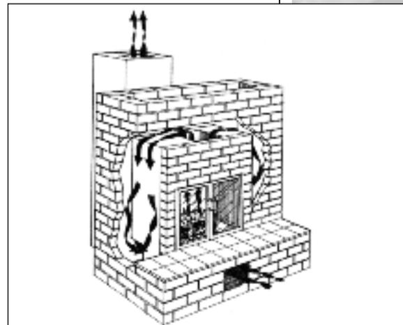
*Masonry heaters are specialized and expensive, but used correctly, they can be efficient and effective. Heat from an intense fire is transferred to the mass of the masonry before being radiated to the room.*
