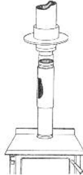
*Certified double-wall flue pipes have a stainless steel inner liner and a sealed or vented outer shell. These pipes cost more than single-wall pipe, but last longer and produce a more stable assembly. Double-wall pipes can normally be placed much closer to combustible materials than single-wall pipe.*
