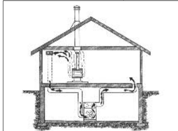
*A central furnace fan operating on low speed can slowly circulate the air in the house and distribute the heat from the stove to other areas. Used continuously, this approach causes increased electrical consumption for the house.*
