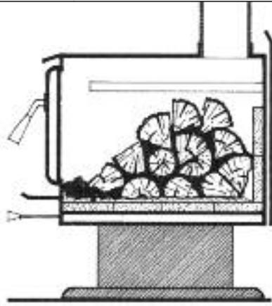
*Rake the charcoal towards the front of the stove where the combustion air enters. Place the pieces of wood on and behind the coals. Open the air inlets fully and leave them open until the pieces of wood are well-charred. This illustration shows the arrangement of pieces for an extended fire.*
