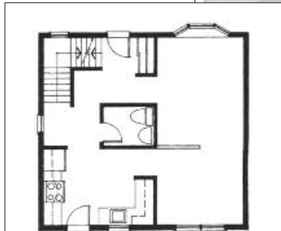
*Houses with an open plan design, where there are few walls to separate rooms on the main floor, can usually be heated effectively with a space heater.*
