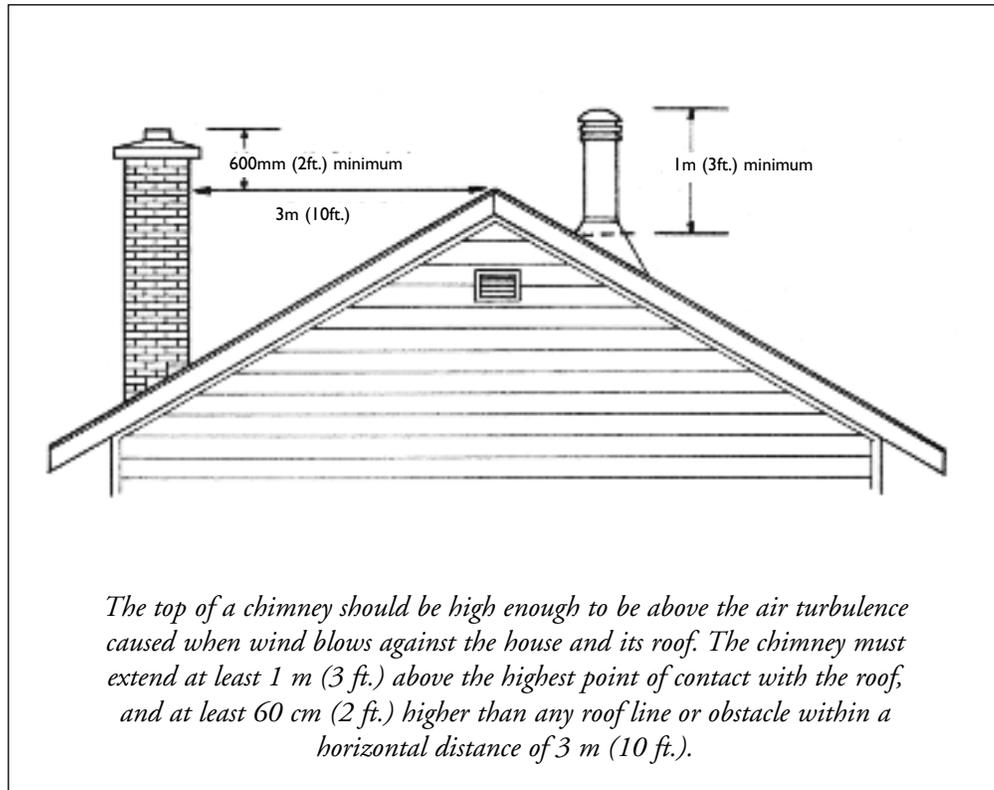
backdraft allows cold air and odours to flow down the chimney, through the appliance and into the room. A backdrafting chimney also makes it hard to build a fire without getting smoke in the house. Chimneys that run up through the house benefit from being enclosed within the warm house environment. Inside chimneys produce stronger, more reliable draft and do not cold backdraft.
